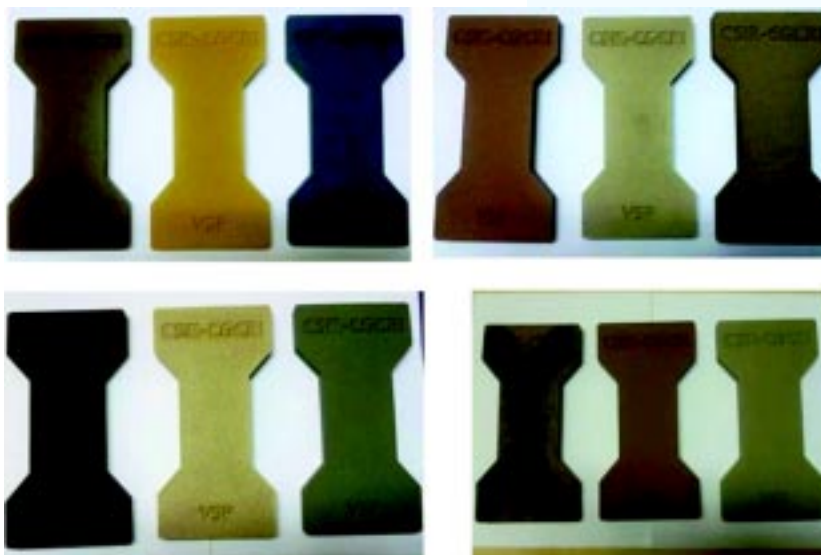
Pavement specimens developed from solid wastes of steel produced by RINL-VSP
