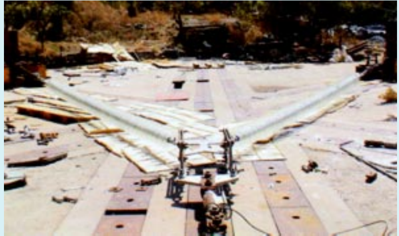
Testing of 800 kV Single "V" Glass Insulator for M/s SEDIVER, France
