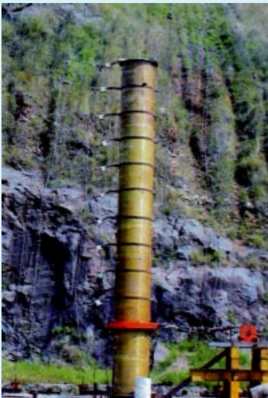
Testing of Glass Fibre Reinforced Plastic (GFRP) Mast for Indian Space Research Organisation (ISRO)
