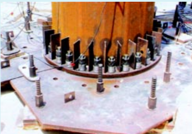
Instrumented foundation bolts
