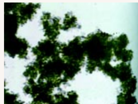
TEM image of platinum nanoparticles (~2nm)
