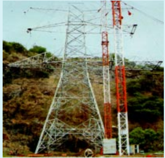
400 kV D/C Tower Type “SE-90” tested for M/s Dubai Electricity & Water Authority, Dubai
