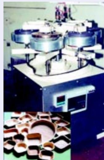
A view of the continuous bioplate-making machine, and finished bioplates/saucers
