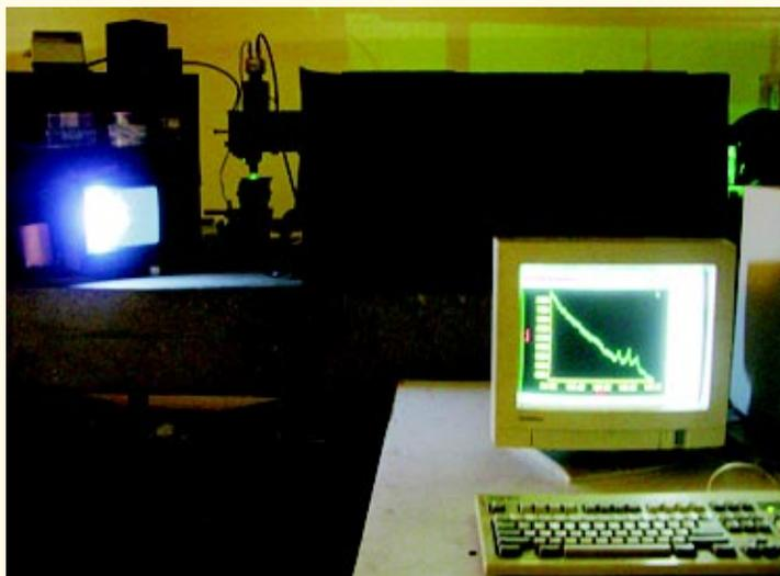
Figure 1: A low-cost Raman Spectrometer with Micro Raman attachment
