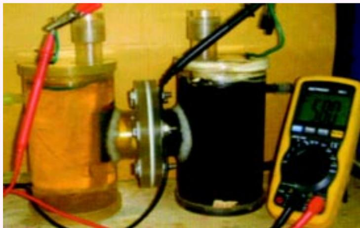
Microbial fuel cell (MFC) [dual chambered; K<sub>3</sub>Fe(CN)<sub>6</sub> cathode] treating chemical wastewater during the production of bioelectricity
