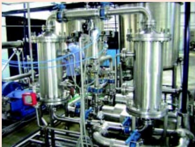
A view of the Membrane Processing Unit at Integrated fruit juice processing plant, Litan, Imphal — the plant was set up by CFTRI for MATA Foundation
