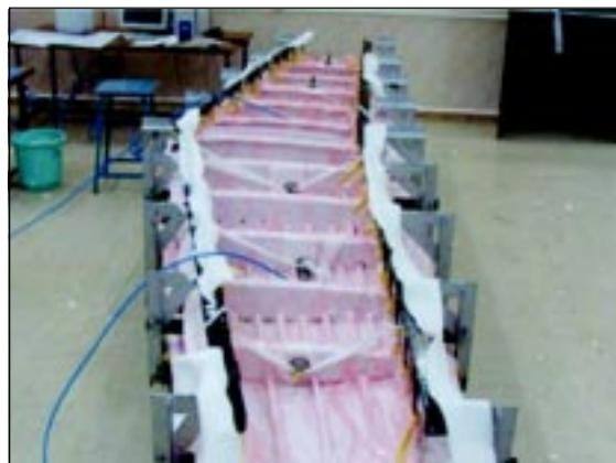
Part bagged before the autoclave
