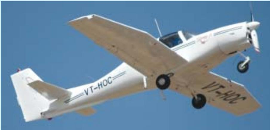
systems. First impression from looking at the HANSA-3 is that the relatively high aspect ratio wing, tapering back to the tips, will give the aeroplane good performance from modest power output, and good glide performance, with nice handling as a bonus. Entry to the cockpit is easier than it may appear, and very comfortable once inside. Controls fall easily to hand. At close to MTOW the HANSA's take-off and climb performance, while modest, is certainly better than expected, and
