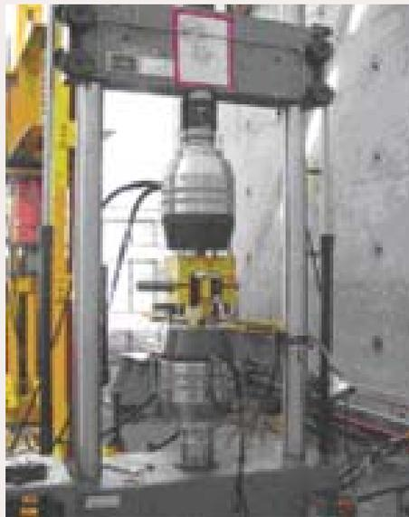
Fatigue testing of 5 HP water pump crankshaft (SERC)
