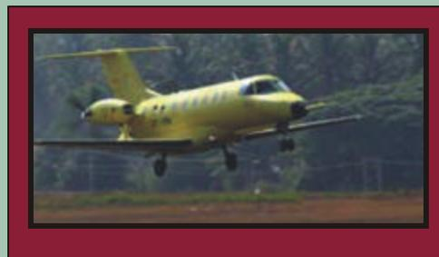
Several improvements have been made in design of the second prototype. The most important one among these is the incorporation of two higher power engines PT 6A-67A of 1200 hp each in PT2 in place of PT6A-66 of 850 hp each used in PT1 and new propellers of larger diameter. This is particularly done to meet the stringent climb gradient requirements under one engine failure condition as stipulated by Federal Aviation Regulations 25 (FAR-25) of USA, the certification standard for *SARAS*.
