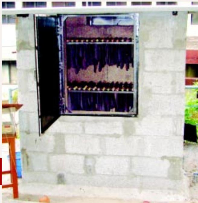
A view of the Fixed type RFNC Rubber Sheet Drier constructed with hollow cement bricks
