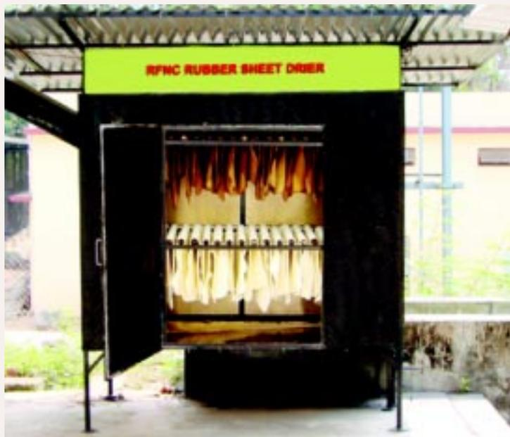
A view of the portable type RFNC Rubber Sheet Drier made with M.S. angles, flats and bamboo plywood
